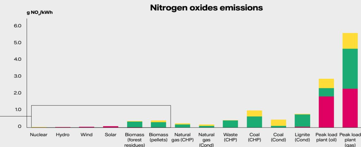
Figure 4. Emissions of nitrogen oxides from a lifecycle perspective, for different electrical power sources.
