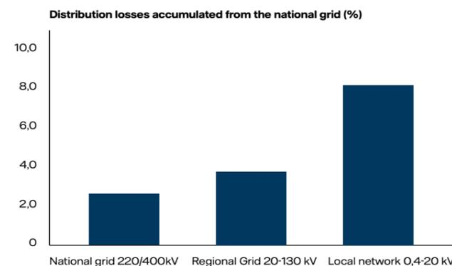
Figure 10. Average distribution losses at different voltages in Sweden.
