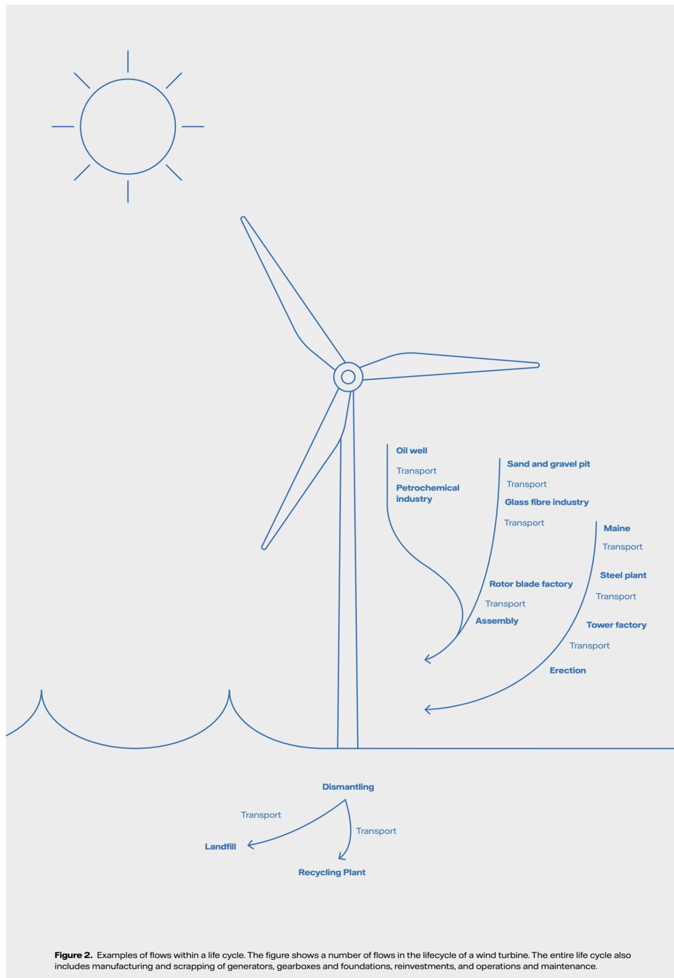
**Figure 2.** Examples of flows within a life cycle. The figure shows a number of flows in the lifecycle of a wind turbine. The entire life cycle also includes manufacturing and scrapping of generators, gearboxes and foundations, reinvestments, and operations and maintenance.
