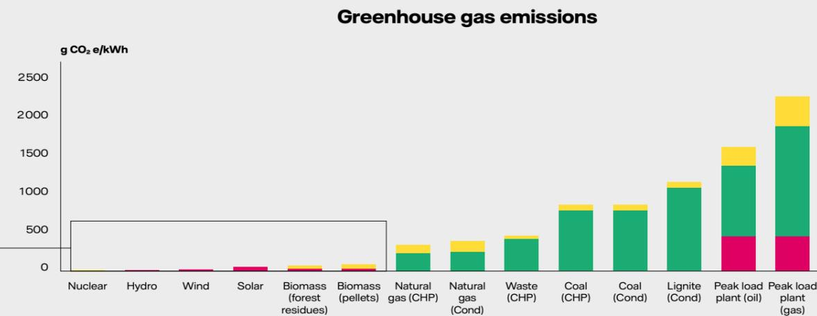
Figure 3. Emissions of fossil greenhouse gases (carbon dioxide equivalents) from a lifecycle perspective, for different electrical power sources.
