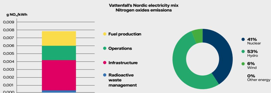
Figure 8. The figure shows energy sources and nitrogen oxides emissions connected to the different life cycle stages.
