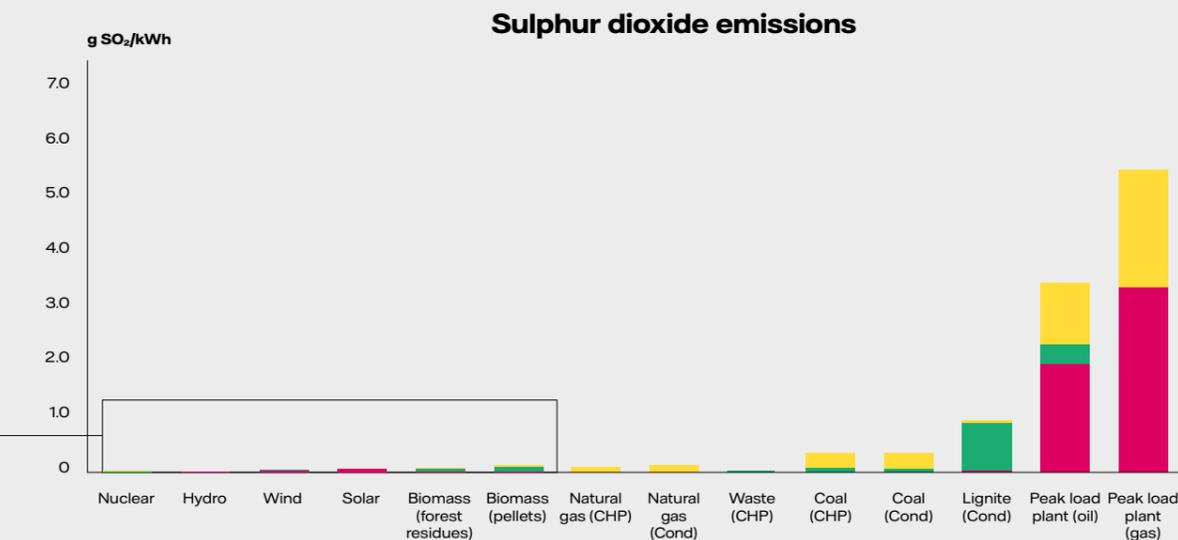
Figure 5. Emissions of sulphur dioxide from a lifecycle perspective, for different electrical power source
