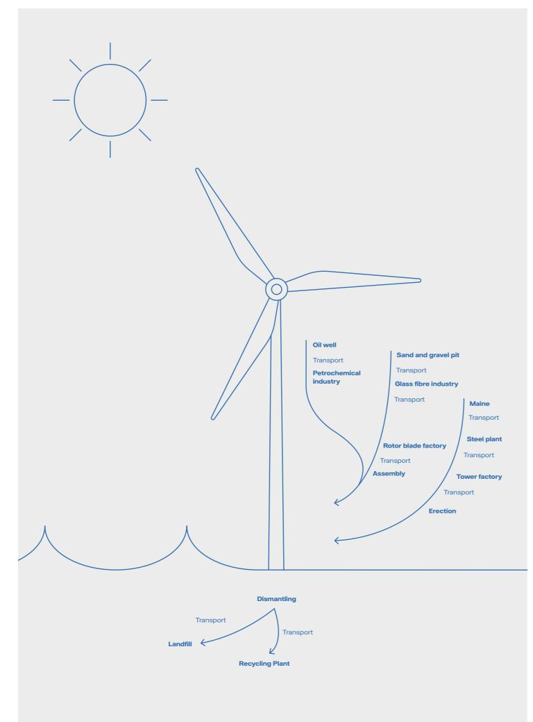
Figure 2. Examples of flows within a life cycle. The figure shows a number of flows in the lifecycle of a wind turbine. The entire life cycle also includes manufacturing and scrapping of generators, gearboxes and foundations, reinvestments, and operations and maintenance.
