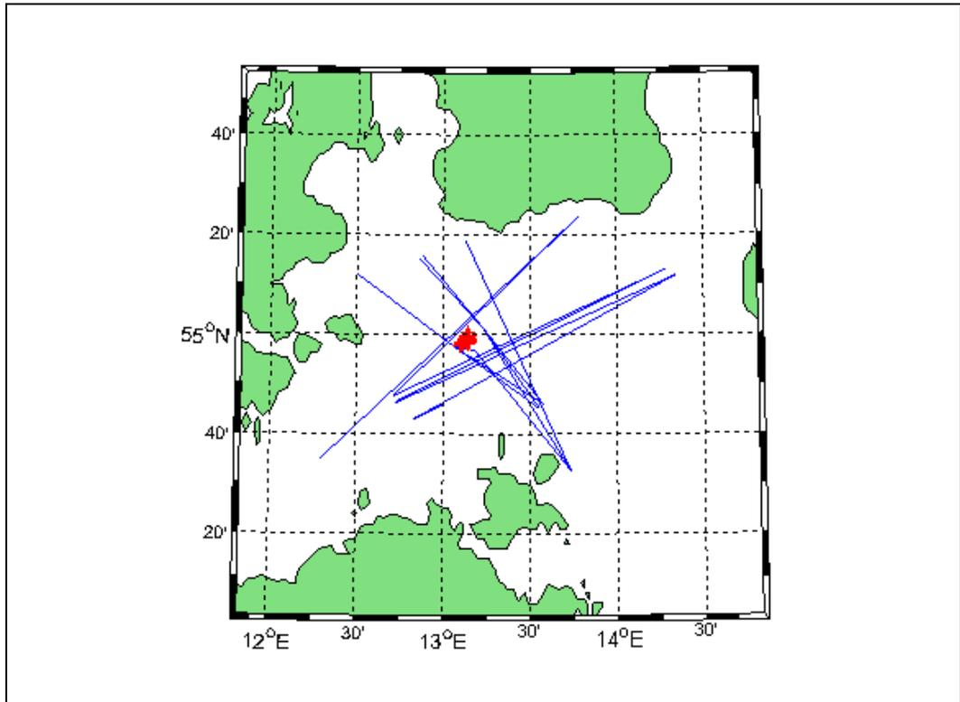
Figure 5.1. MARIN's wind farm and shipping lanes for powered collision (illustrated by SSPA's calculation program).
