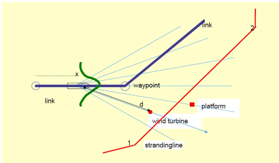
Figure 3.3. MARIN's model: Collision opportunity times Navigational Error Rate (NER). Source: van der Tak (2005a).
