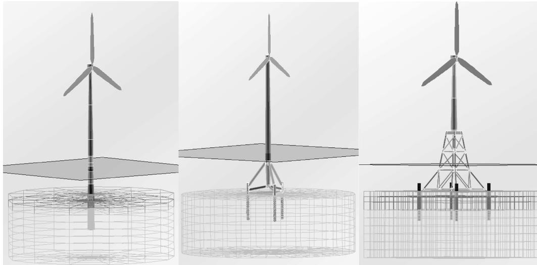
Figure 3.7. Offshore wind turbine support structures considered by Biehl and Lehmann (2006B). Figure taken from Biehl and Lehmann (2006B).
