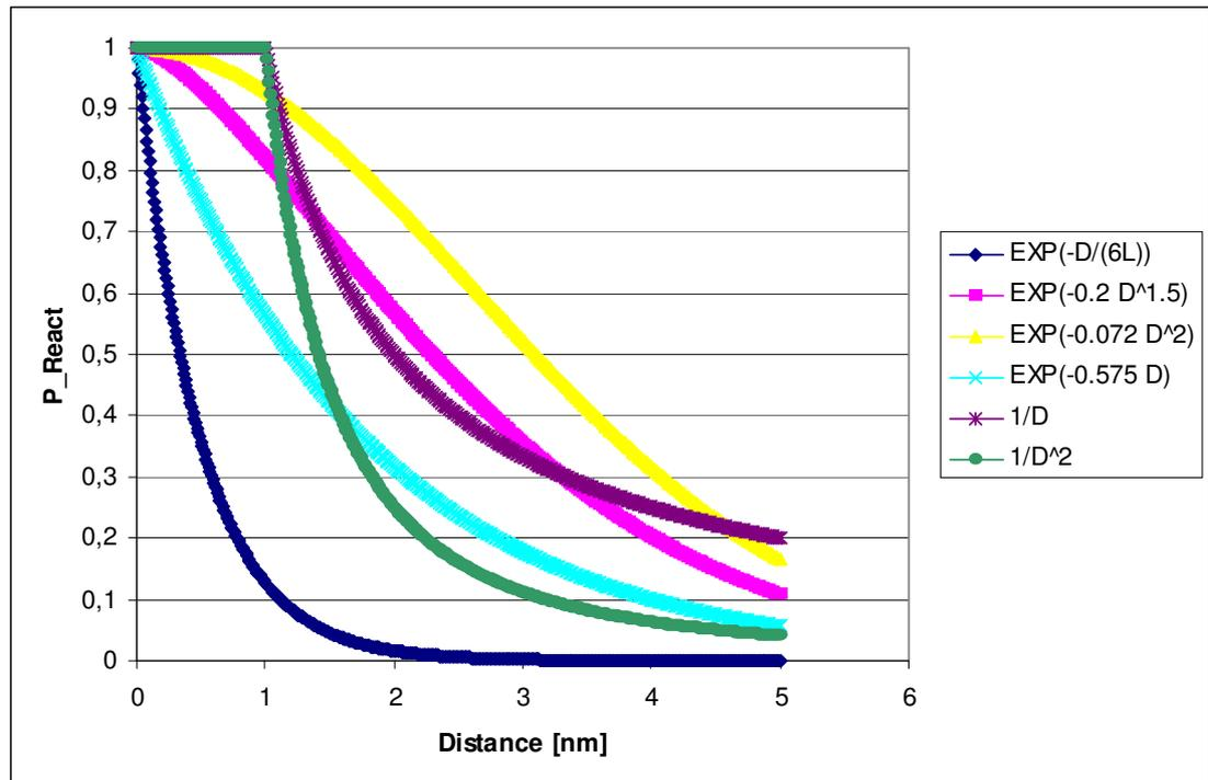
Figure 5.9. Weightings for offshore platforms presented by MARIN (all curves except for  $\exp(-D/(6L))$ ) (van der Tak and Glansdorp (Year unknown)).  $P_{\text{react}}(x) = \exp(-D/(6L))$ , where  $L$  = ship length, is suggested in the literature to be used together with the causation factor (Fujii and Mizuki 1998). The ship length ( $L$ ) is assumed to be 150 m.
