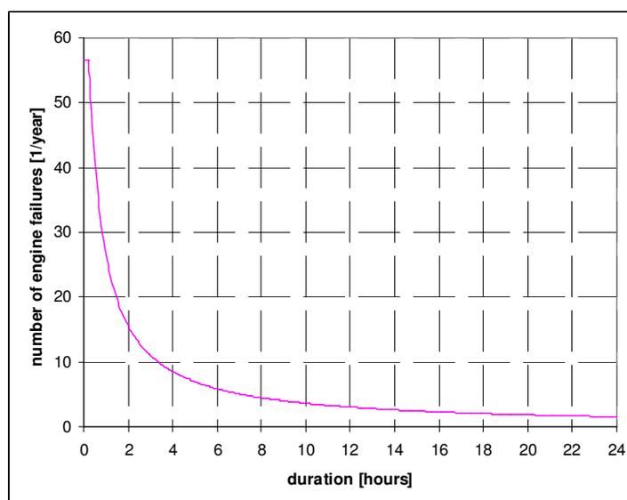
Figure 3.5. “Self repair function” used by MARIN with 56.5 drifters per year.
