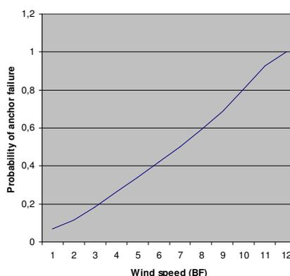
Figure 5.7. Probability of anchor failure used in SSPA’s simulations of GL’s calculations for Kriegers Flak.
