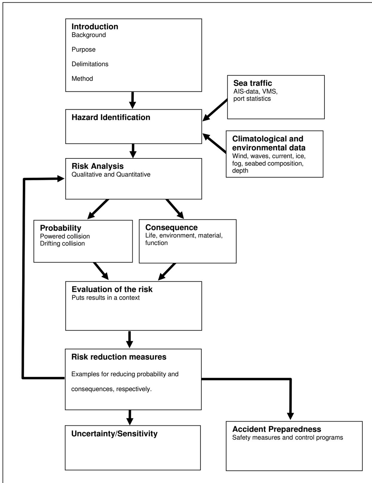
Figure 2.3. SSPA's procedure for assessing navigational risks associated with offshore wind farms.
