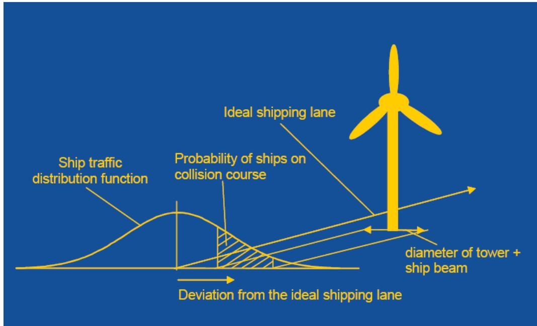
Figure 3.2. Illustration of general probability calculation model based on Gaussian distribution of ship traffic along a fairway. Collision course times causation factor. Source: van der Tak (2005a).
