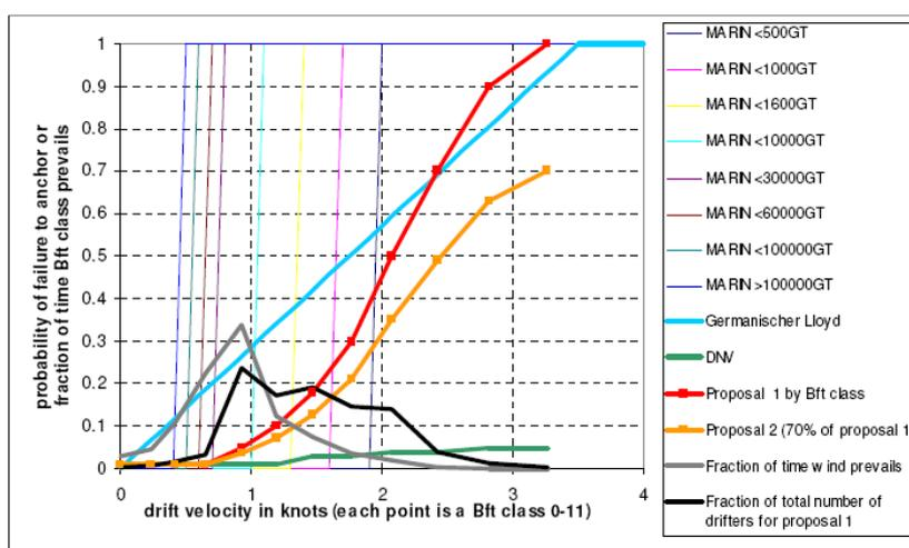
Figure 5.6. Probability of anchor failure (SAFESHIP 2005).
