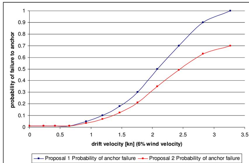
Figure 3.6. Probability of failure to anchor (data from SAFESHIP 2005).
