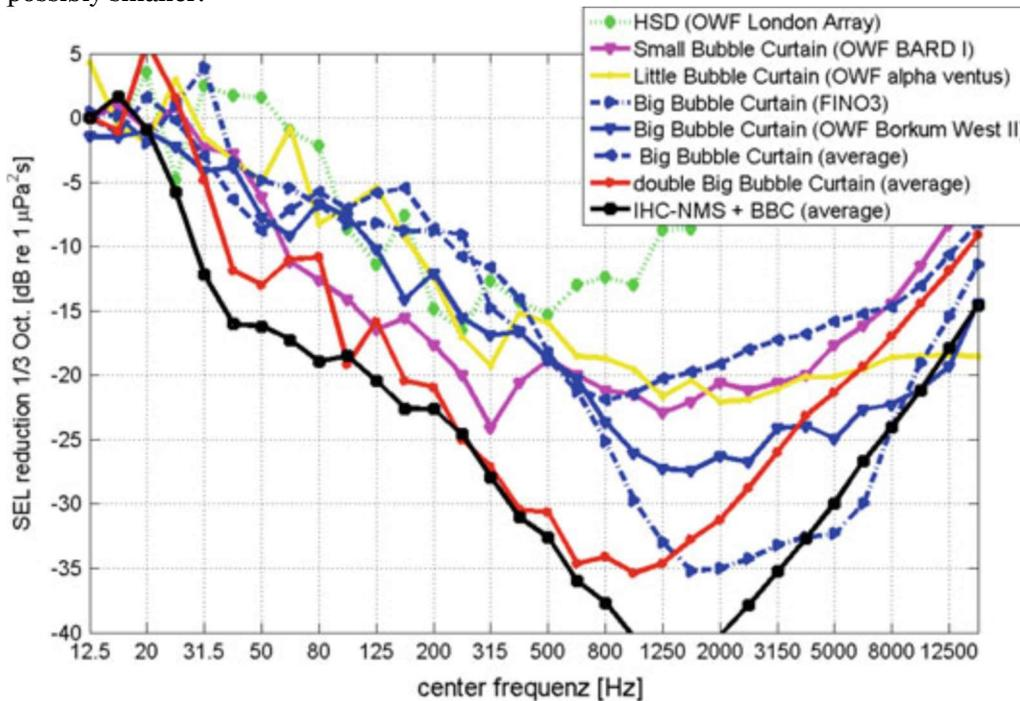
In addition, it should be noted that although there is additional attenuation to gain from employing multiple technologies at the same time, the combined effect is less than the simple sum of the attenuation of the individual systems in isolation. Examples can be found in the data from the DanTysk offshore wind farm (Dahne et al., 2017) and in the
