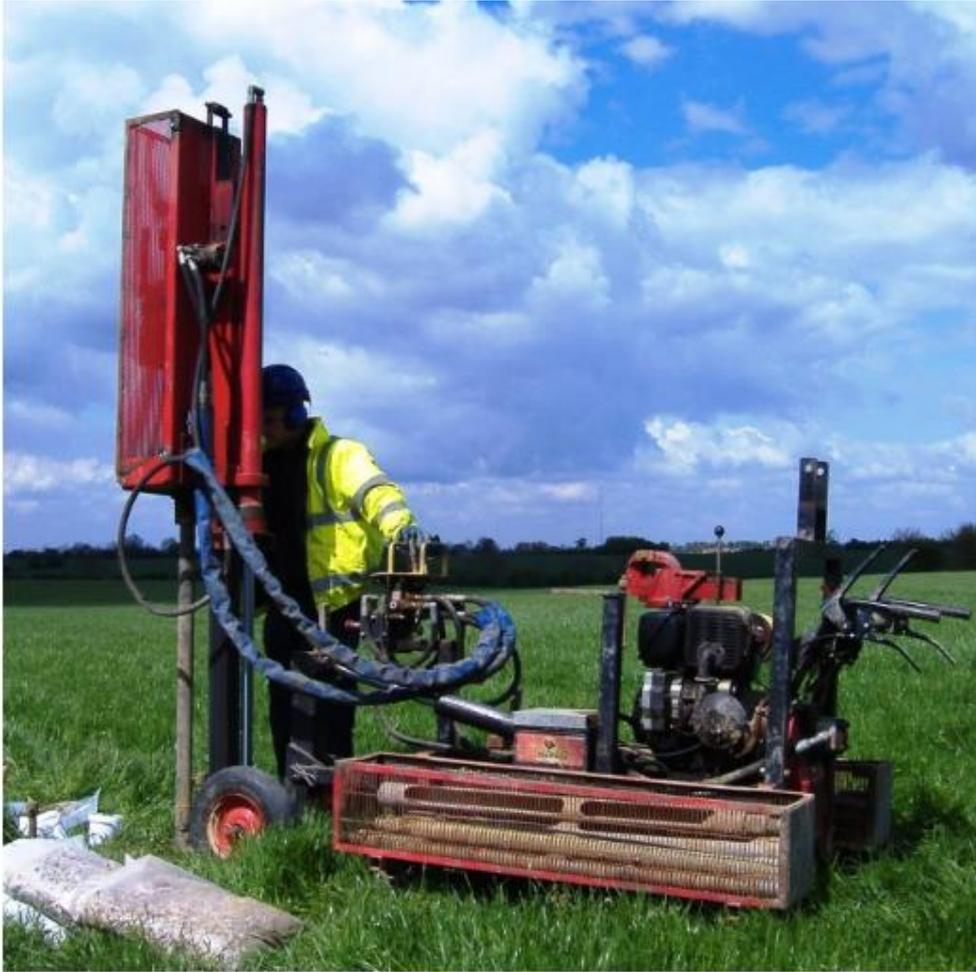
Fig 3. Window sample drilling rig
