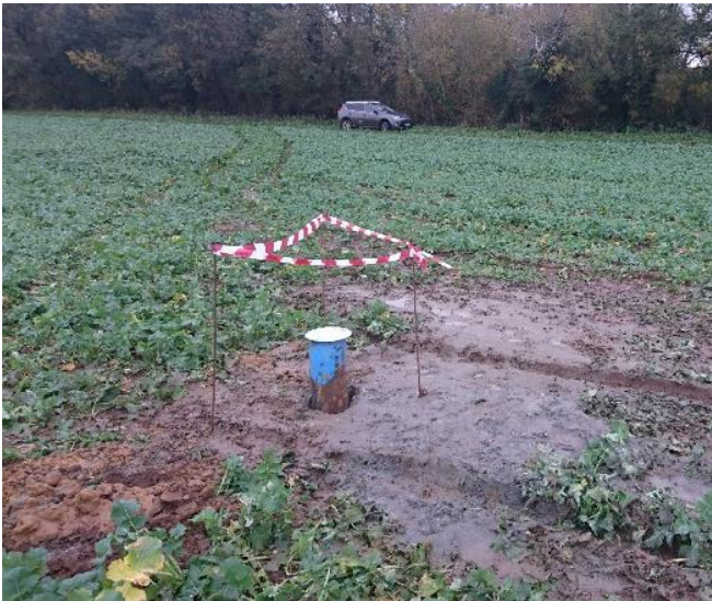
Fig 2. Picture of a ground water and gas monitoring station
