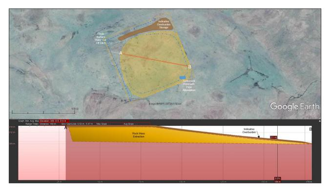
Figure 4.4: Indicative BP3 Working Area – 1.6Ha - Rock Volume ~ 21,000m<sup>3</sup> Overburden Volume ~ 4,900m<sup>3</sup>
