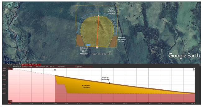
Figure 4.3: Indicative BP2 Working Area - 1.1Ha - Rock Volume ~ 45,000m<sup>3</sup> Overburden Volume ~ 3,300m<sup>3</sup>
