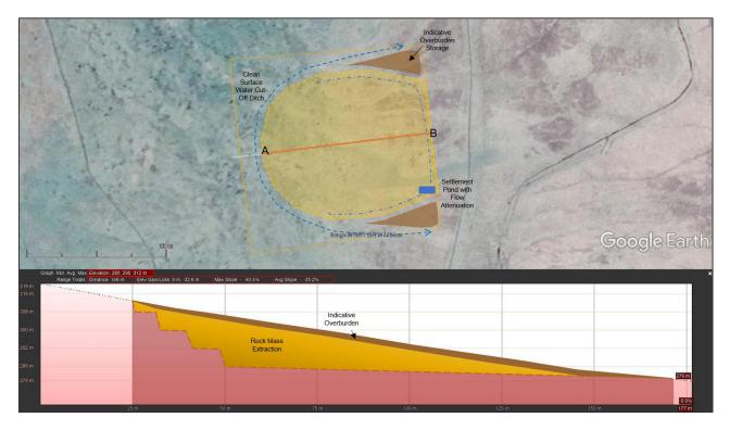
Figure 4.2: Indicative BP1 Working Area –1.4Ha – Rock Volume ~ 65,000m<sup>3</sup> Overburden Volume ~ 4,100m<sup>3</sup>
